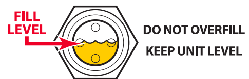
FIGURE 57. CHECK OIL LEVEL AT SIGHT GLASS
