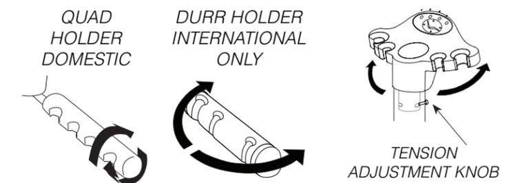
The assistant's holder tension adjustment knob allows operator to easily alter the holder position. Turn adjustment knob counter-clockwise to decrease tension; clockwise to increase tension. Tighten tension adjustment knob to secure assistant's holder into preferred position.
