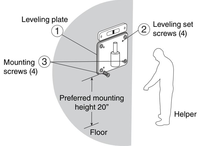
1. Mount large 16" x 18" plate on wall. If wall mount plate is not needed, proceed to step 2.
