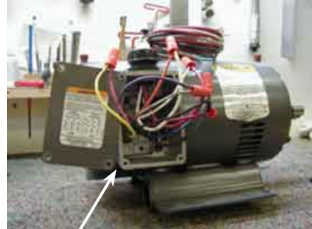
Motor junction Box
