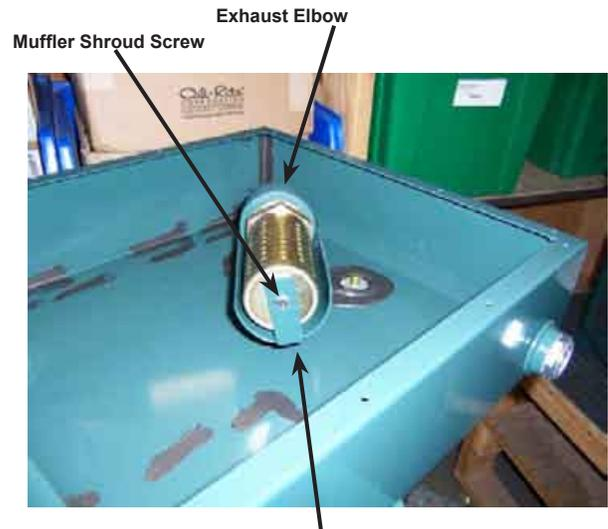
Muffler Shroud: Tip slightly as shown
