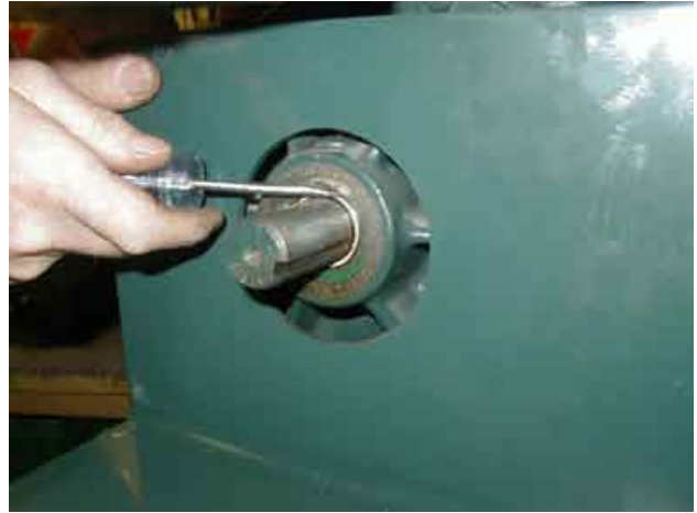
Outer Seal Removal
