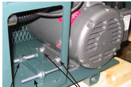
Belt Tension Bolt
